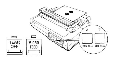
**Caution:** The short tear-off feature can only be used with the built-in tractor feeding system.
